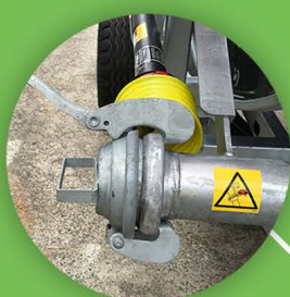
Water Pipe Inlet Plug
