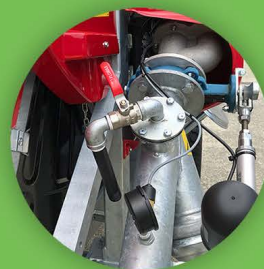
Water Inlet Drain Valve
