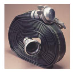
Features unique "through-the-weave" one piece construction comprising a circular woven high tenacity polyester reinforcement totally encapsulated in a tough vulcanised rubber cover and lining. The integral woven construction imparts extremely high tensile strength to withstand all practical loading conditions.
